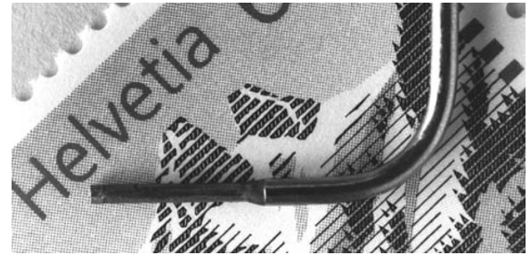
Figure 11. Tip of one-sensor Pitot probe of 0.84 mm diameter manufactured mainly by electric discharge machining (Kupferschmied et al 1994). The sensor chip (sensitivity of typically 90 mV bar -1 at 5 mW excitation power) is located one tip diameter behind the tap to improve the accuracy of the total pressure reading and reduce the angular sensitivity. The limitations were shown to be related to assembly, electric connections and sealing.
