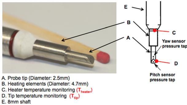
**Fig. 2 FRAP-HT heated probe schematic and temperature measurement locations**
