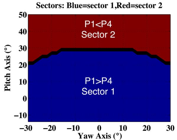
**Fig. 4 FRAP-HTH extended calibration section's schematic for Ma = 0.3**
