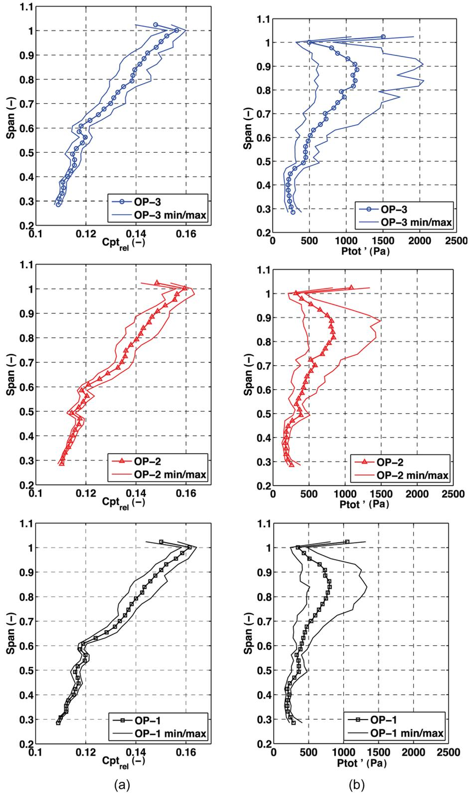
Fig. 9 (a) Time-averaged spanwise distribution of  $Cpt_{rel}$  and (b) time-averaged RMS of  $P'_{tot}$  (Pa) at rotor exit of L-1 stage for OP-3, OP-2 and OP-1 with their respective minimum and maximum values obtained from the time-resolved data
