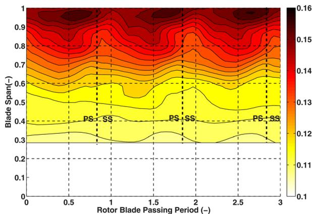
**Fig. 10 Time-resolved  $Cp_{t,rel}$  (—) at rotor exit of L-1 stage for OP-3**
