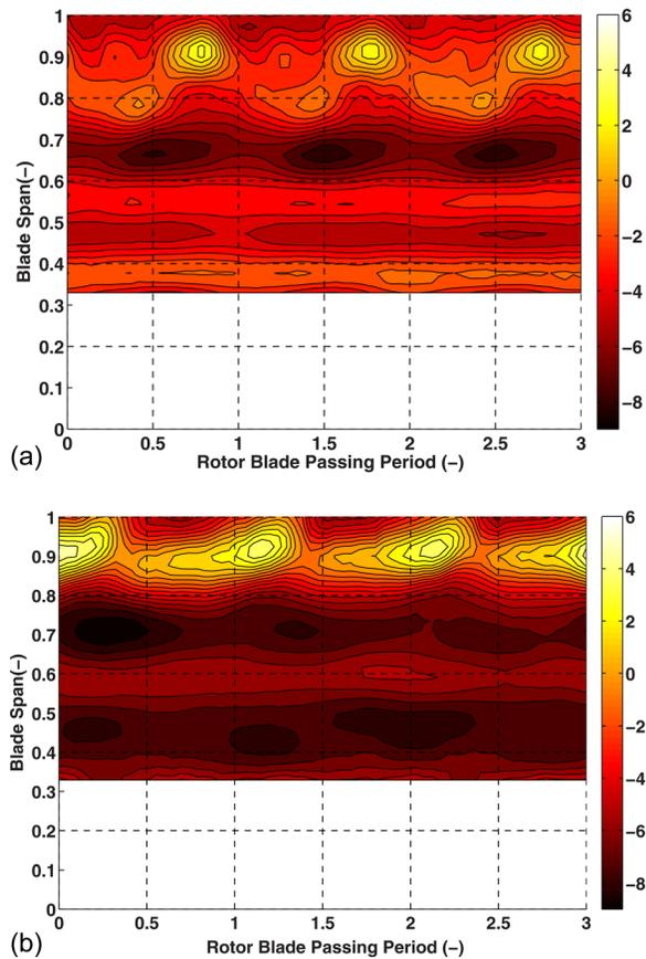
**Fig. 18** Time-resolved relative flow yaw angle (deg) at rotor exit of L-0 stage for (a) OP-3 and (b) OP-2 (relative to blade metal angle)
