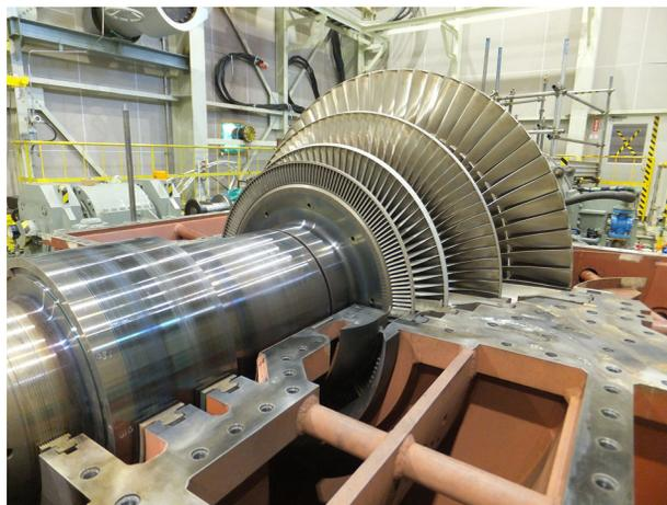
Fig. 5 LP steam turbine test facility where FRAP-HTH measurements were conducted
