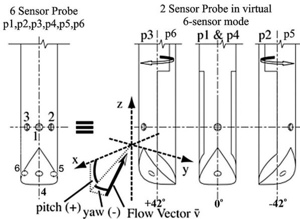
**Fig. 3 Measurement concept in virtual six-hole mode with two-hole probe**
