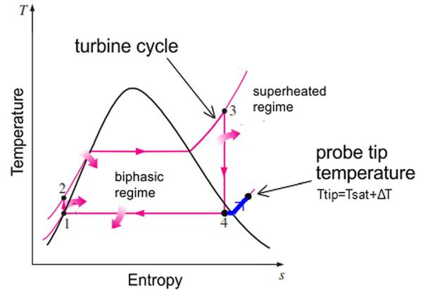
Fig. 1 T–S diagram with steam turbine operating cycle and the respective probe tip operating temperature
