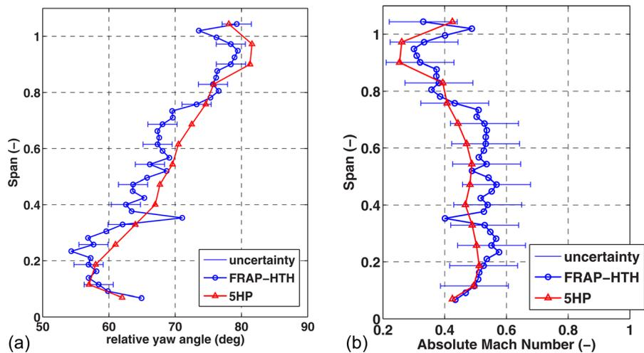
Fig. 8 Relative flow yaw angle (a) and absolute Mach number (b) of 5HP and FRAP-HTH probes at rotor exit of L-0 stage
