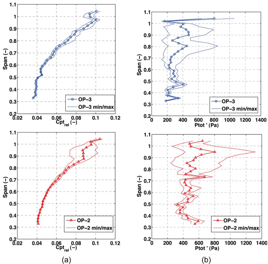
Fig. 15 Time-averaged spanwise distribution of  $C_{pt,rel}$  (a) and time-averaged  $P'_{tot}$  RMS (Pa) (b) at rotor exit of L-0 stage for OP-2 and OP-3 with their respective minimum and maximum values obtained from the time-resolved data
