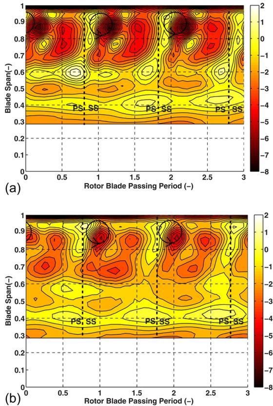
**Fig. 12 Time-resolved relative yaw flow angle (deg) at rotor exit of L-1 stage for (a) OP-3 and (b) OP-1 (relative to blade metal angle)**
