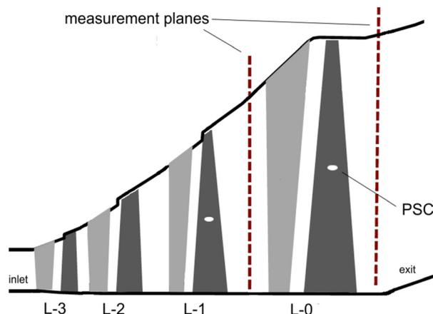
Fig. 6 Schematic of the steam turbine test facility with the respective probe measurement locations
