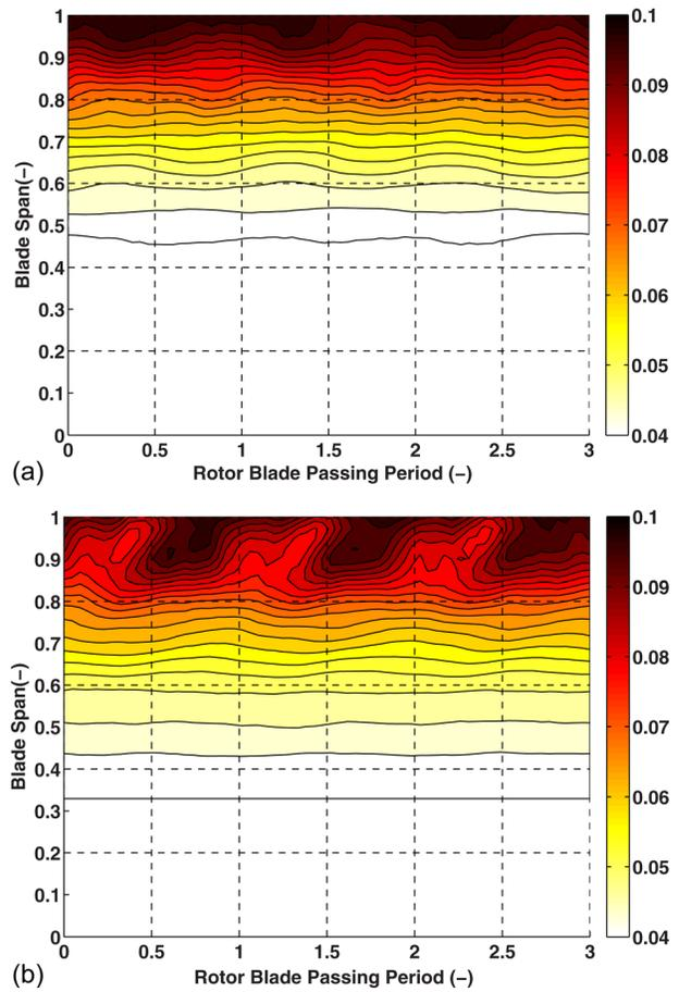
**Fig. 19** Time-resolved  $C_{pt,rel}$  (—) at rotor exit for (a) OP-3 and (b) OP-2
