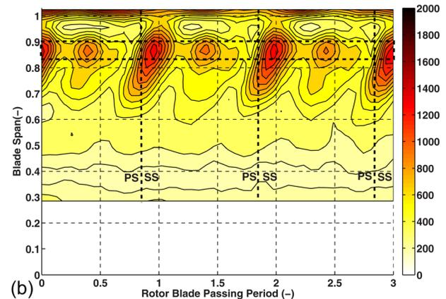
**Fig. 11 Time-resolved RMS of  $P'_{tot}$  (Pa) in stationary frame of reference at rotor exit of L-1 stage for (a) OP-3 and (b) OP-1**
