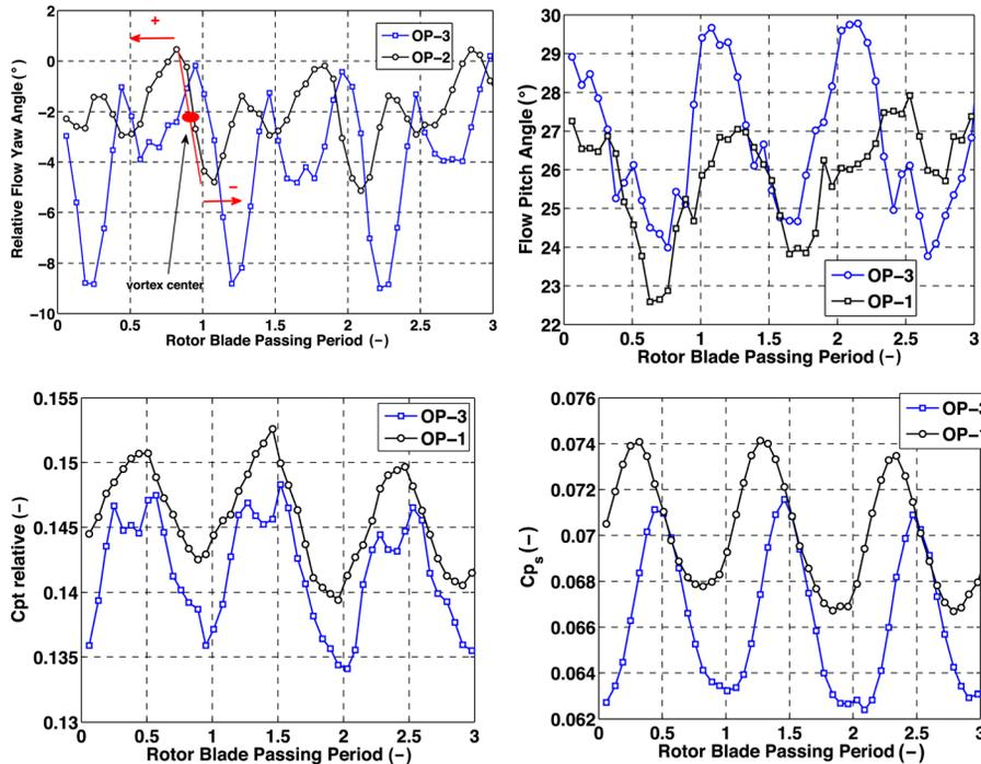
**Fig. 13 Unsteady relative flow yaw and pitch angles, relative total and static pressure coefficients at 86% span for OP-3 and OP-1**
