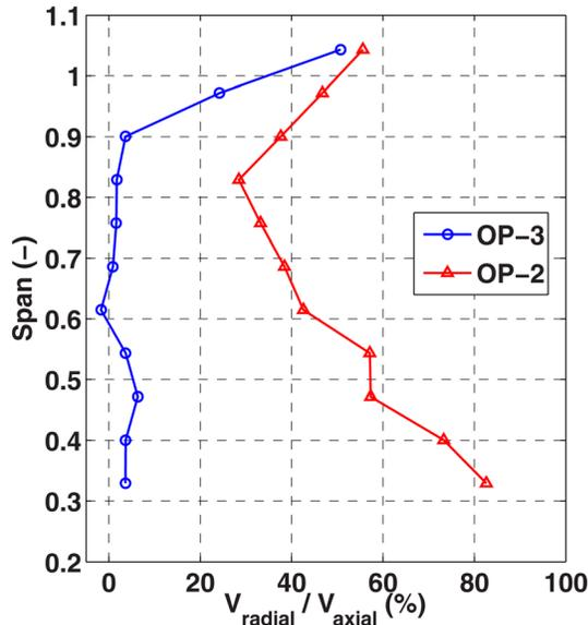
Fig. 16 Time-averaged spanwise distribution of  $V_{\text{radial}}/V_{\text{axial}}$  at exit of L-0 stage
