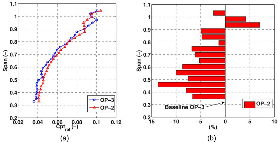
Fig. 14 Time-averaged spanwise distribution of the  $C_{pt}$  in relative frame of reference for two operating conditions (a) and difference in  $C_{pt,rel}$  between OP-2 with OP-3 (b)
