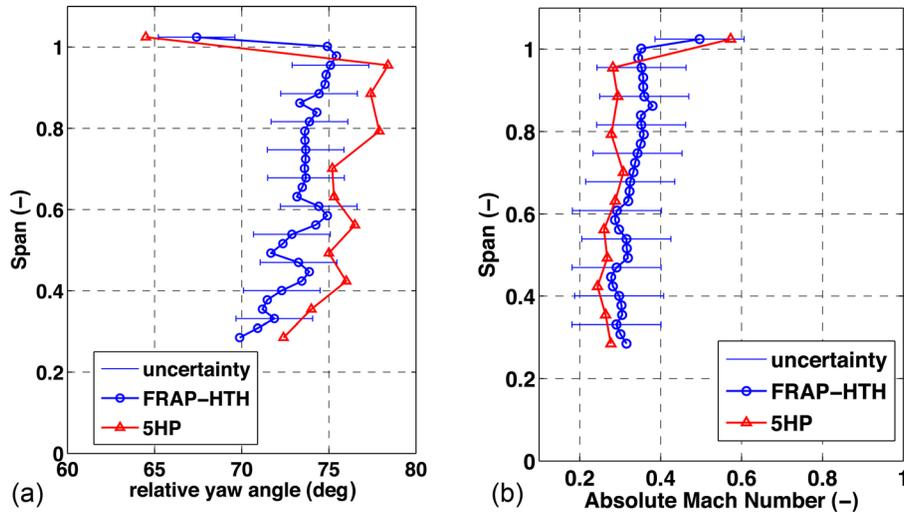
Fig. 7 Relative flow yaw angle (a) and absolute Mach number (b) measured by the 5HP and FRAP-HTH probes at rotor exit of L-1 stage
