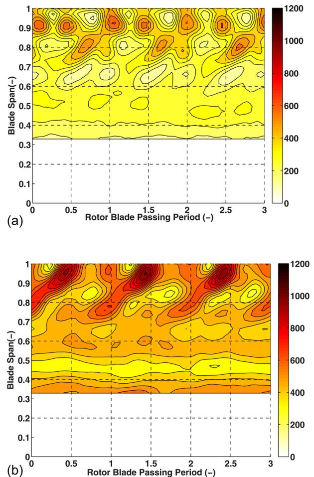
Fig. 17 Time-resolved RMS of  $P'_{\text{tot}}$  (Pa) in stationary frame of reference at rotor exit of L-0 stage for (a) OP-3 and (b) OP-2
