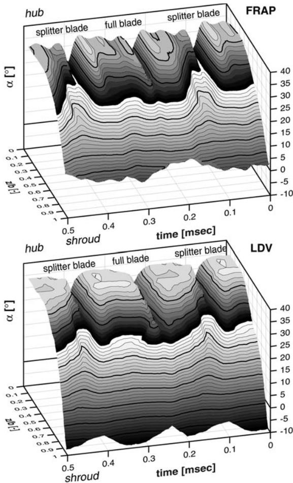
**Figure 29.** Comparison of the ensemble-averaged flow angle distribution at the impeller exit, measured with fast-response probes (top) and LDV (bottom); running conditions of the stage:  $\text{Mu} = 0.75$ , best point.
