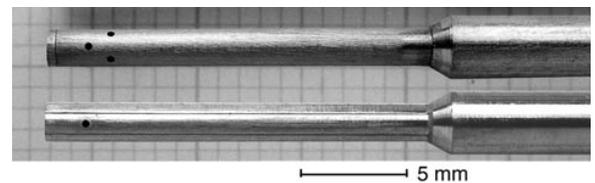
**Figure 12.** Tips of a one- and a three-sensor probe of 1.80 mm diameter (Kupferschmied 1998). The sensor chips are located behind the taps, as in figure 10, with the diaphragm turned towards the interior to avoid damage due to particle impact on the chip's active side. This kind of probe has been successfully operated over several hundred hours.
