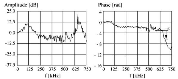
**Figure 14.** Amplitude and phase response of a miniature pressure sensor in a recessed cavity determined in a shock tube (Gossweiler 1993). The first peak reveals the natural frequency of the cavity (90–105 kHz, depending on the probe type), and the second peak the sensor diaphragm eigenfrequency (650–850 kHz, depending on sensor type).
