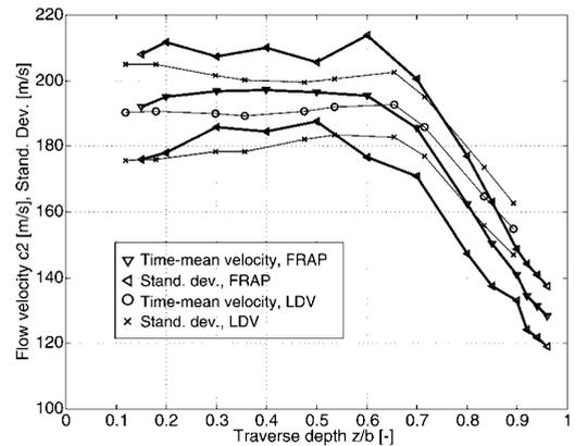
**Figure 30.** Time-mean absolute mean velocity and standard deviation of the FRAP and LDV measurements. Note the stretched velocity scale.
