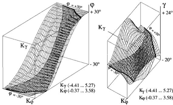
**Figure 20.** Calibration surfaces  $\varphi (K_\varphi, K_\gamma)$  and  $\gamma (K_\varphi, K_\gamma)$  of a cylindrical four-hole probe at  $M = 0.2$  (Kupferschmied 1998). Due to the large angular range required for fast-response measurements, the coefficient surfaces show a rather complicated shape.
