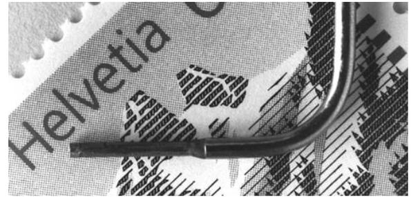
**Figure 11.** Tip of one-sensor Pitot probe of 0.84 mm diameter manufactured mainly by electric discharge machining (Kupferschmied *et al* 1994). The sensor chip (sensitivity of typically  $90 \text{ mV bar}^{-1}$  at 5 mW excitation power) is located one tip diameter behind the tap to improve the accuracy of the total pressure reading and reduce the angular sensitivity. The limitations were shown to be related to assembly, electric connections and sealing.
