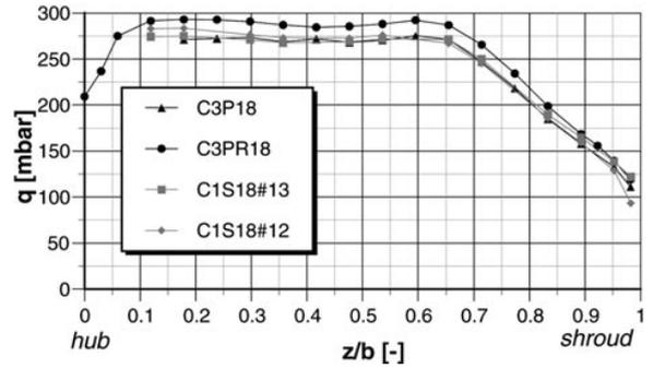
**Figure 27.** Wall-to-wall dynamic head distribution at  $r/r_2 = 1.05$ .
