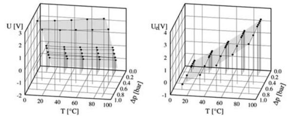
**Figure 6.** Typical output signal  $U$  and excitation signal  $U_e$  of a miniature piezoresistive pressure sensor chip as a function of temperature and pressure (Sensym P788, excitation current 1 mA).
