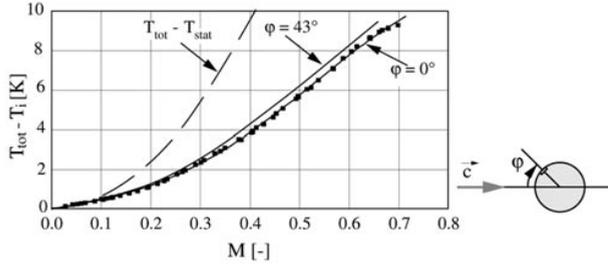
**Figure 18.** Difference between the flow total temperature and the temperature indicated by the probe FRAP C1S18 No 12.
