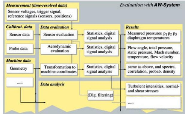
**Figure 24.** Steps of the conversion of measured data.
