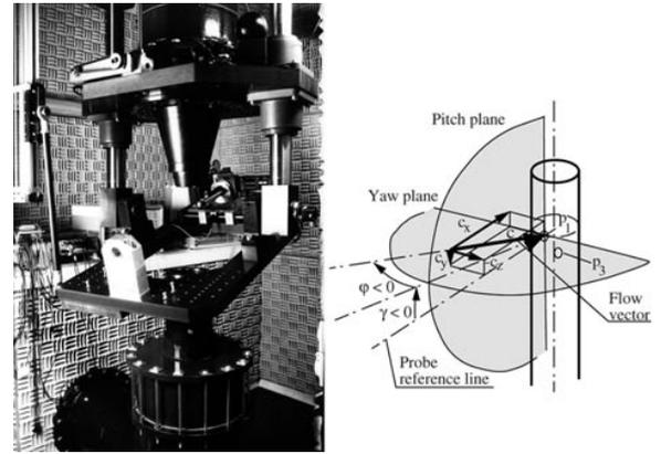
**Figure 16.** Left: vertical-nozzle free jet facility (diameter 100 mm) of the ETH Turbomachinery Laboratory. This dedicated facility has been designed to achieve an accuracy one order of magnitude higher than the accuracy required in the later application.
