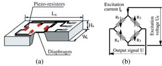
**Figure 5.** (a) Piezoresistive miniature pressure sensor chip (die), typical size  $1.7 \times 0.6 \times 0.2 \text{ mm}^3$ . (b) Schematic of the typical Wheatstone bridge deposited on the diaphragm.
