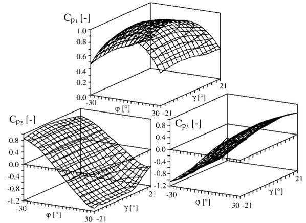
**Figure 17.** Aerodynamic coefficients of a three-hole probe (C3S18P, diameter 1.80 mm,  $M = 0.30$ ). Each mesh node is a calibration point. The frame of reference of the probe is defined in figure 16 (right). The overall repeatability of the  $C_p$  is better than  $\pm 2\%$ .
