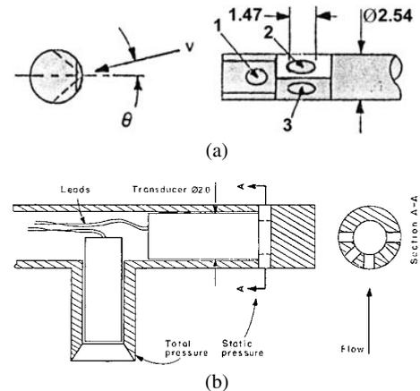
**Figure 2.** Early fast-response probes developed for the MIT Blowdown Compressor Facility (Kerrebrock *et al* 1974). The cylinder probe (a) used for flow field surveys downstream of the rotor was equipped with three surface-mounted silicon pressure diaphragms. The flow field upstream was measured with a total-static fast-response probe (b) containing two standard commercial sensors.
