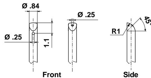
Figure 2: Final probe head design
