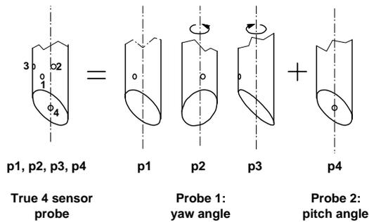
Figure 1: Measurement concept of a virtual 4 sensor probe.
