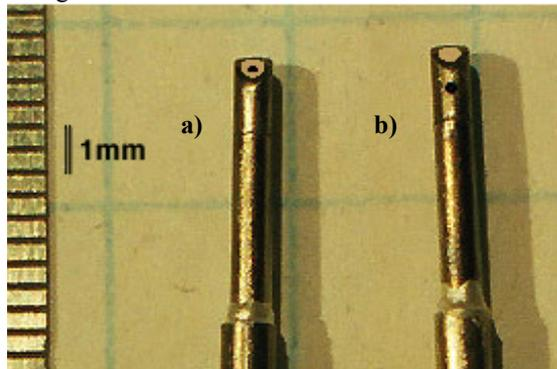
Figure 4: a) pitch angle sensitive probe
