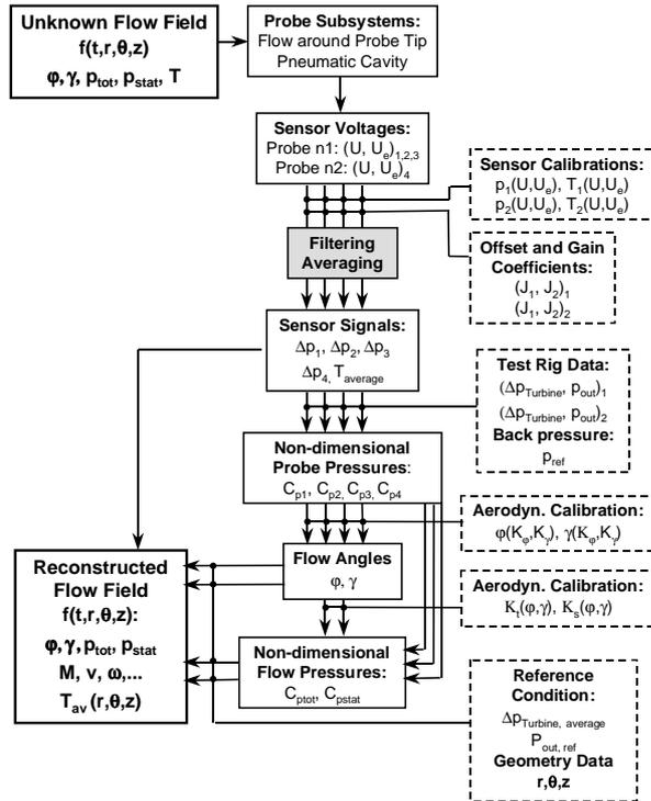
Figure 9: Signal paths from flow to measurement results
