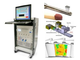
The fast-response aerodynamic probe turn key system is designed to measure the temporal fluctuation of the 3-dimensionnal flow velocity field either in air or steam. The system consists of calibrated fast-response aerodynamic probes delivered with a 2 or 3-axis traversing system and a rack mounted system comprised of a PC, data acquisition boards, probe signal conditioning units.
