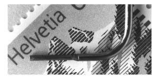
**Figure 11.** Tip of one-sensor Pitot probe of 0.84 mm diameter manufactured mainly by electric discharge machining (Kupferschmied *et al* 1994). The sensor chip (sensitivity of typically 90 mV bar<sup>-1</sup> at 5 mW excitation power) is located one tip diameter behind the tap to improve the accuracy of the total pressure reading and reduce the angular sensitivity. The limitations were shown to be related to assembly, electric connections and sealing.
