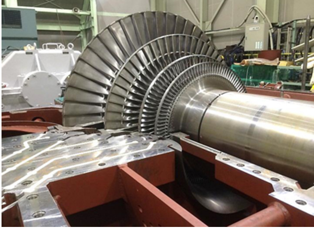
Fig. 3 MHPS' low-pressure steam turbine test facility where FRAP-HTH and FRAP-OB measurements were conducted
