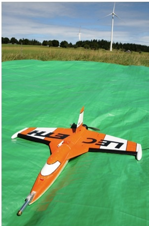
Fig. 3 Instrumented UAV (wingspan, 800 mm) equipped with a seven-sensor fast response aerodynamic probe (diameter, 20 mm)
