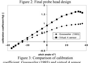
coefficient: Gossweiler (1993) and virtual 4 sensor probe,  $\varphi=0^{\circ}$
