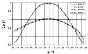
Figure 5: Pressure reading of both probes at 0° pitch angle and two Mach-numbers, M=0.15, 0.3
