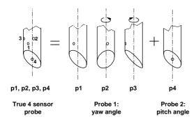
Figure 1: Measurement concept of a virtual 4 sensor probe.
