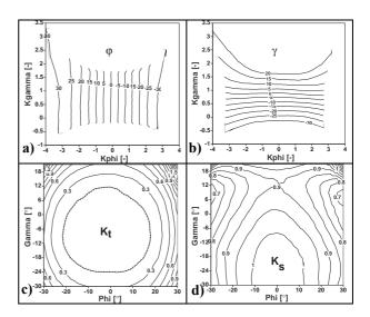
Figure 7: Aerodynamic calibration surfaces:  $\phi$ ,  $\gamma$ ,  $K_t$ ,  $K_s$
