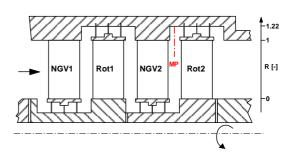
Figure 10: Cross section of the test turbine with measurement position
