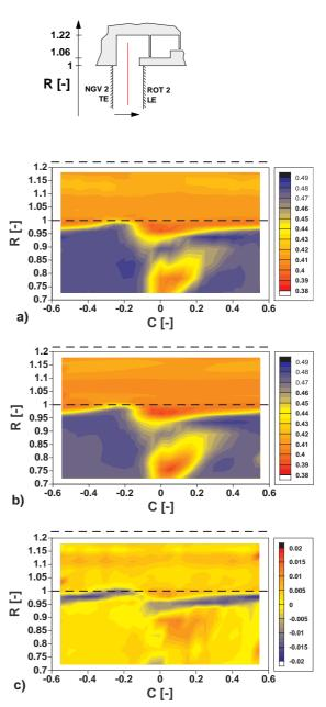
Figure 11: Comparison of non dimensional total pressure C<sub>p</sub>: a) virtual 4 sensor probe, b) 5 hole probe, c) difference a-b
