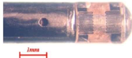
**Fig. 2 Photograph of the tip of the unsteady entropy probe**
