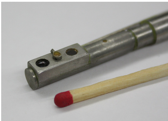
Figure 7. The optical backscatter probe tip.
