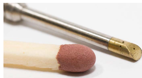
Fig. 8 Cylindrical four-hole probe (FRAP shape) presented with a match for scale comparison
