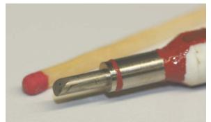
The unique Fast-Response Aerodynamic Probe – High Temperature Heated (FRAP-HT) is designed for unsteady 3-dimensionnal flowfield measurements in wet steam environment. The FRAP-HTH is a robust measurement tool that has been used in the last stage of industrial low-pressure steam turbine facilities under high wetness fraction and high Mach number conditions.
