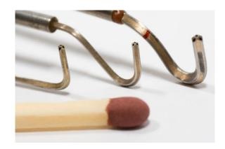
miniature pneumatic 5-hole probes are designed for steady 3-dimensionnal flowfield measurements. These probe are robust and routinely used in industrial and academic facilities.
