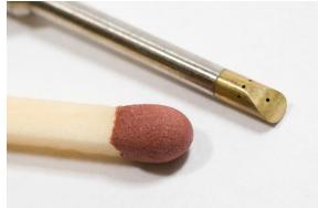
The miniature pneumatic 4-hole probes are designed for steady 3-dimensionnal flowfield measurements. These probe are robust and routinely used in industrial and academic facilities.
